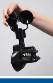
The GS026 cup design is extremely flexible, dramatically reducing wind cup breakage.
