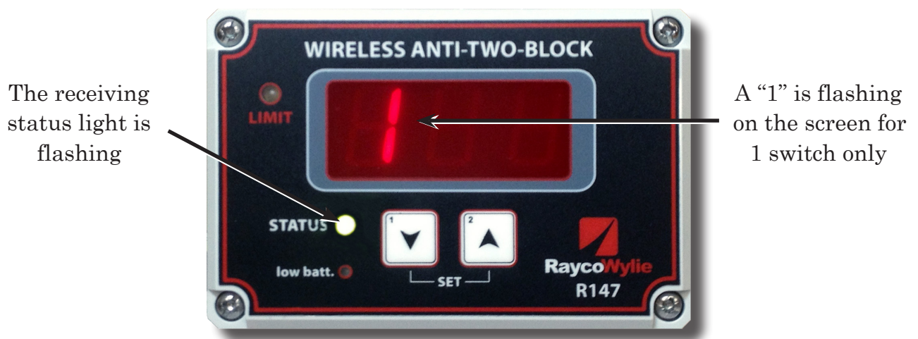
Picture 3: R147 Waiting for transmission from the ATB switch
