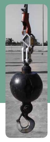
The "quick slip" design allows you to simply slip the LSI Skip Frame over the load cell and secure it into place utilizing the existing load cell adaptor plate pin. This quick, no-nonsense installation saves valuable time on the job site.
