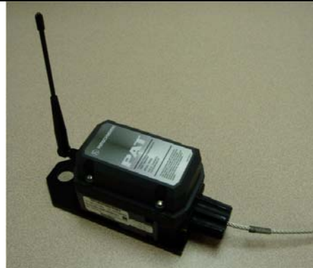
031-300-060-593 Radio A2B transmitter assembly 031-300-050-537 Battery cover (includes screws, gasket, and cardboard tubes)
