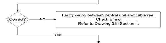
Measure angle signal analog input module between test point MP0(AGND) and X1:4 (ang sig). The measurement should be between 0.5-4.5v. 0.5v(500mv) with the boom at 0° or 4.5v with the boom at 90°.
