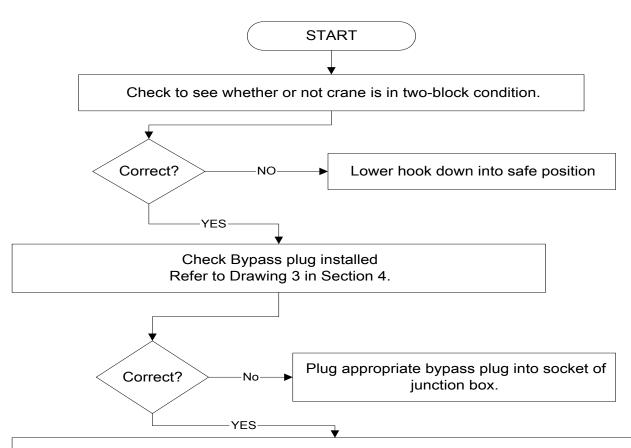
Turn power off or disconnect wire from connection board X1:31 in central unit. Remove the bypass plug and measure the resistance at the boom nose box between terminals 1 and 6 with a ohmmeter. This checks the function of the Anti-Two Block switch.
