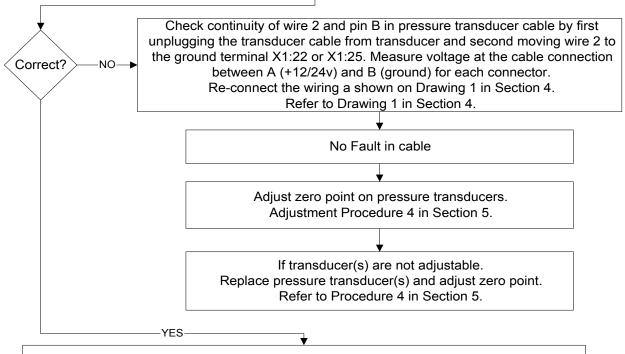
Measure pressure transducer signals on the analog input module between test points: Piston Side, MP0 (ground) and X1:1.
